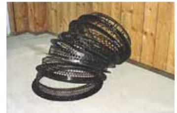
**How short should the straw be? Try all six screens to determine which is most suitable.**
